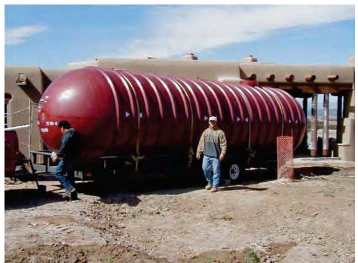
Figure 3-4: A 10,000 gallon tank like the one shown above must be delivered to the site on a flatbed trailer.
